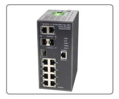
The ICE810G SNMP managed compact switch supports web based management and advanced features such as RMON, IGMP snooping, 802.1Q VLAN tagging, 802.1D spanning tree, Port Security. The advanced management features together with the rugged environment capabilities make the ICE810G switch a powerful solution for out-door installation and for daisy chain and ring topology networks usually deployed for security surveillance and monitoring applications.
